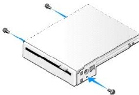
3. Align the screws on the drive with the bracket slots in the computer, and gently position the drive until it clicks into place.
