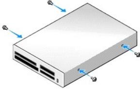
4. Align the shoulder screws on the media card reader with the shoulder screw slots, and gently slide it into the bay until it clicks into place.
