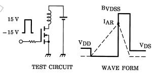
$$\begin{aligned} &R_G = 25~\Omega \\ &V_{DD} = 90~V,~L = 17.4~mH \end{aligned} \quad E_{AS} = \frac{1}{2} \cdot L \cdot I^2 \cdot \left( \frac{BV_{DSS}}{BV_{DSS} - V_{DD}} \right)$$
